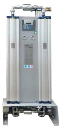
Two towers are filled with adsorbant materials. They are designed to filter  $H_20$  molecules by sieving.  $H_20$  molecules which adhere to the surface of adsorbent material can be easily separated by the interaction of molecular forces from where they are hold. While the first tower dries the incoming air, the second tower is regenerated with the reverse-direction regenerative air. This is a physical reaction and can be repeated countless times
